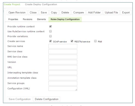
Figure 124: Defining rules deploy configuration settings
